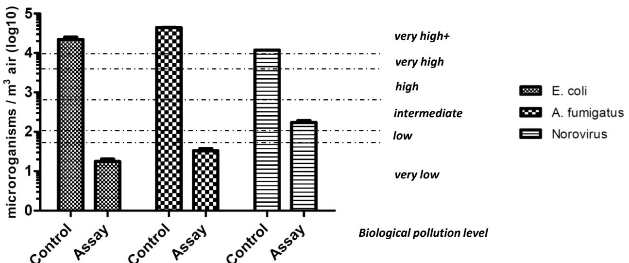
**Figure 1.** Efficiency of AERAMAX PRO AM IIIS system after 13min and 42s functioning time corresponding to 18 theoretical circulation of chamber biological pollutants.
