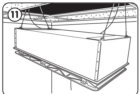
Raise the unit until the top of the housing is just below the grid.
