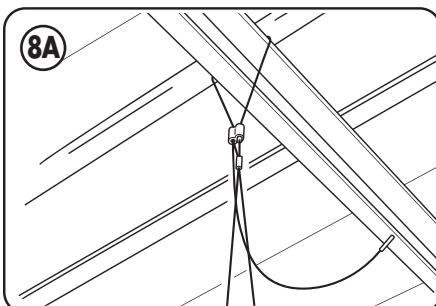
Loop open end of cables through intended support or hardware.
