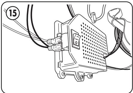
Ensure power switch located on the power supply is in the off position before proceeding with connecting any wires.
