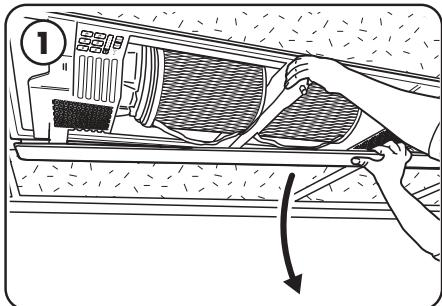
Open the door by depressing the latch button and pulling down on the door.
