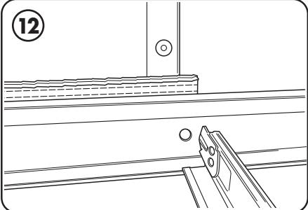
Check below units for visible gaps. If needed, add centering blocks between unit and grid. Trim out as desired.
