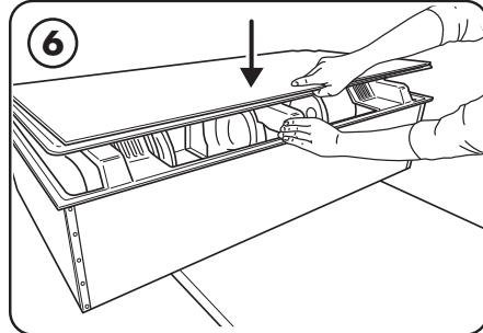
Close the door until a click is heard. Depending on type of ceiling, attach proper mounting hardware above installation area per local regulations for supporting a 92 lb (42kg) fixture. Ideally the mounting locations would be at the four corners of a 23" x 46" rectangle.
