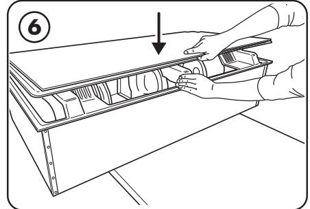
Close the door until a click is heard. Depending on type of ceiling, attach proper mounting hardware above installation area per local regulations for supporting a 92 lb (42kg) fixture. Ideally the mounting locations would be at the four corners of a 23" x 46" rectangle.
