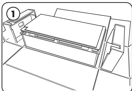
Before beginning installation, ensure that a qualified electrician has run a 120V circuit to the installation area. Remove unit from packaging and stage on a tabletop or other surface under or near installation area with door facing upwards.
