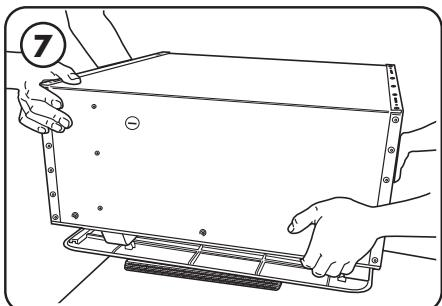
Lift and rotate unit before setting door-side down on the provided trays. Determine which electrical knockout will be used and remove it.
