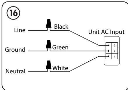
Have a qualified electrician connect the ground, line, and neutral to fixture per local electrical codes.
