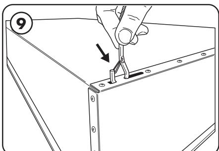
Secure the hooks from the provided aircraft cabling to the housing through the mounting holes.
