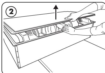
Open unit door by depressing the latch button and pulling upward. Have one person hold the door open while filter and hardware are removed.
