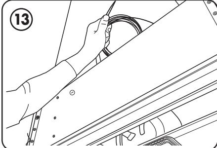
Coil and wrap remaining cable out of the way.
