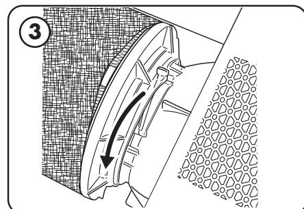
Disengage the filter clamp lever until a click is heard.
