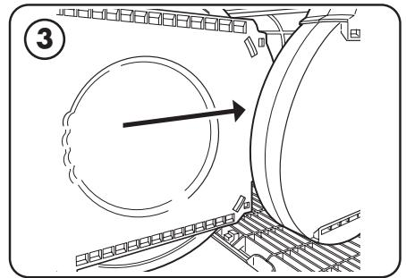
Remove new filter from protective bag and properly dispose of bag.
