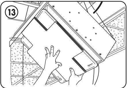
Rotate and lift all the way through the grid until fixture can be straightened above the ceiling grid ensuring bottom panel is not damaged.
