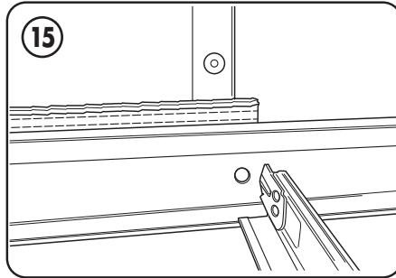
Check below unit for visible gaps. If needed, add centering blocks between unit and grid. Trim out as desired.
