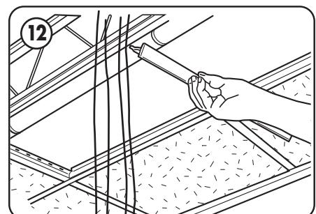
If you have not yet, remove the adjacent cross-tee, tilt fixture about 45° upward toward the grid's long tees.
