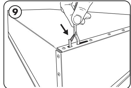
Secure the hooks from the provided aircraft cabling to the housing through the mounting holes (P7).
