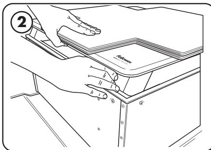
Open unit door by depressing the latch button and pulling upward. Have one person hold the door open for the next few steps or the hinges can be damaged.
