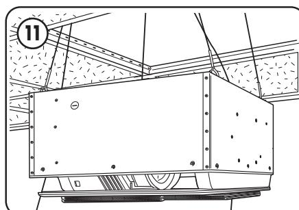
Raise the fixture to about 1-2 feet below the ceiling grid on the cables.
