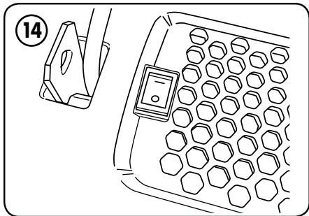
Flip power switch to the ON ("I") position.
