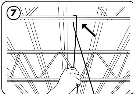
Depending on type of ceiling, attach proper mounting hardware above installation area at proper distances per local regulations for supporting a 45lb (21kg) fixture.
