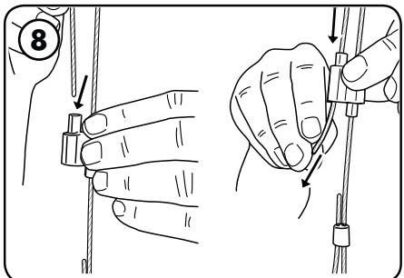
Loop open end of cables through intended truss.
