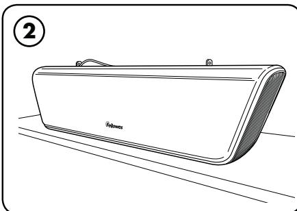
Remove unit from packaging and stage on temporary support trays on a tabletop or other surface under or near installation area.
