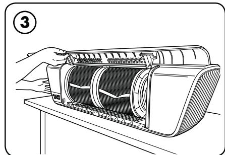
Open unit door by peeling back the tape as needed and gently pulling outward on the bottom of the door panel.
