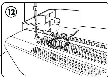
Coil and wrap remaining cable out of the way. Do not trim excess cable lengths.
